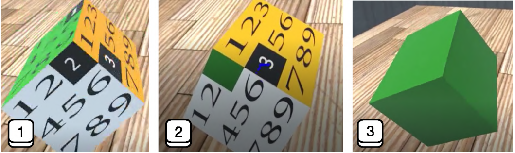
Fig. 3. In the usability study, participants were asked to enter predefined passwords. The digits and their order were visualised using white digits on a black background (i.e., 1, 2, 3 and 4) as shown in (1) and (2). Upon selection of four digits, the entire cube turned green if the authentication was successful as shown in (3), or red if the input was incorrect.
