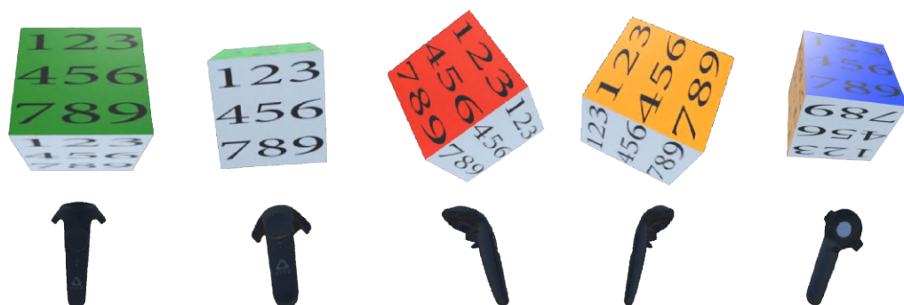
Fig. 1. We propose RubikAuth, a novel authentication scheme for immersive virtual reality. Users wearing a head-mounted display and holding a controller in each hand are presented with a 3D cube that they can manipulate (i.e., rotate) to authenticate in VR. The figure shows how controller's pose affects the cube. To authenticate, users point at each desired digit and surface using either a) eye gaze, b) head pose, or c) tapping with the right-hand controller, and confirm using the left controller's trigger button. Through three user studies, we assess RubikAuth's usability, memorability, and observation resistance under three realistic threat models. Findings of our usability study reveal the advantages of coordinated 3D manipulation and pointing on a manipulable 3D object in VR. Our in-depth security study emphasises the importance of considering advanced threat models to accurately assess a system's security.
