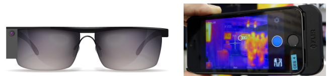
Figure 1: Examples of how thermal cameras are becoming more portable, discrete and usable in everyday scenarios Left: Illustration of possible future wearable thermal camera, based on current research prototype [10]. Right: Thermal camera smartphone add-on [13].
