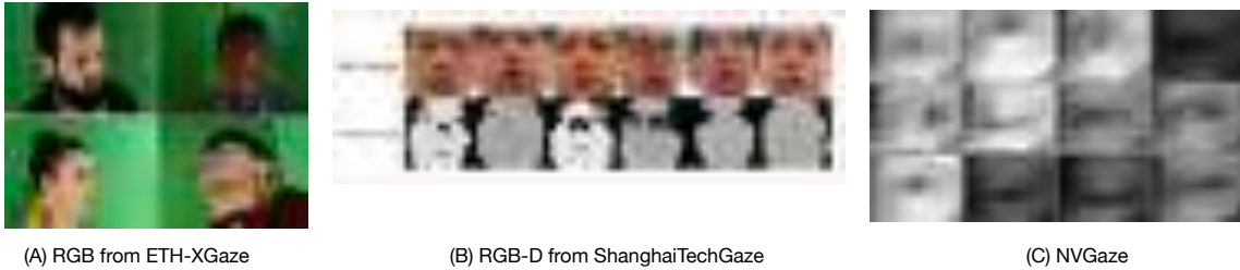
Fig. 2. Examples of images from cameras that are readily integrated into handheld mobile devices, and can be used for gaze estimation: (A) RGB [268], (B) RGB-D [155], and (C) IR [124]
