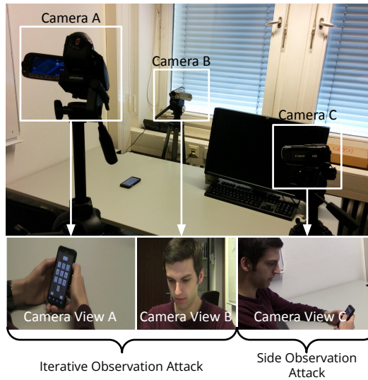
Fig. 3. The figure shows the camera setup used for both usability studies. To prepare videos for the subsequent security studies, we recorded users using three cameras. Camera A recorded the phone screen (phone-view) to observe the touch input. Camera B recorded the participant's face (eyes-view) to observe the eye movements. Camera C simultaneously recorded the screen and the user's eyes (side-view). The views from Camera A and B were used to evaluate the schemes' resistance to iterative observation attacks, whereas the view from Camera C was used to evaluate resistance to side observation attacks.
